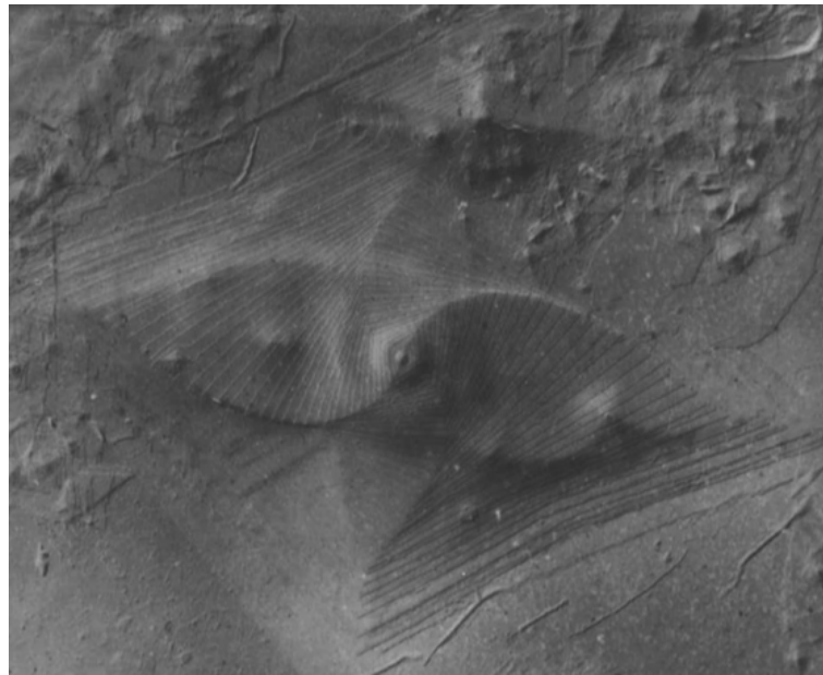
Figure 2.10: Remarkable electron micrograph of a stack of chain folded single crystals of PE that have all nucleated from a central screw dislocation site; the picture has been taken from a presentation by [33] that did not unfortunately mention any scale
